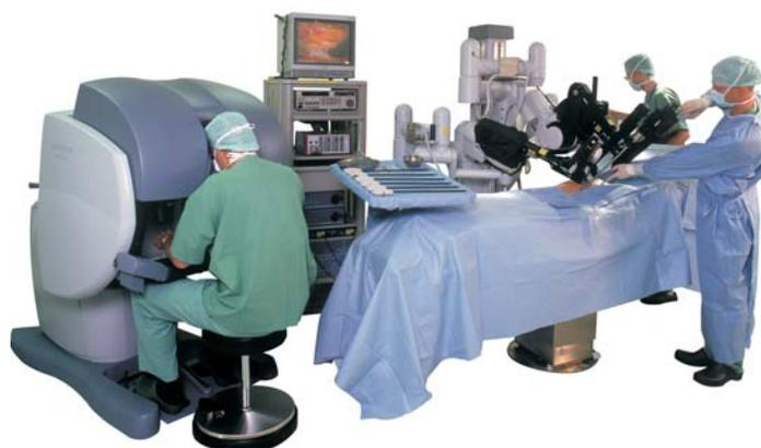
The da Vinci Surgical System - Surgeon is seated at the console at a short distance from the patient-side cart with the four interactive robotic arms and the vision system. A robotic arm uses instruments that provide seven degrees of freedom.
